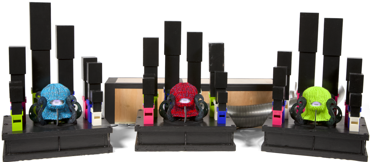
Figure 1: Three miniature pipe organs consisting of three colorful Dr. Squiggles octopus-shaped robots, the three wind chests that they are on, 24 organ pipes, and one air supply in the rear.
