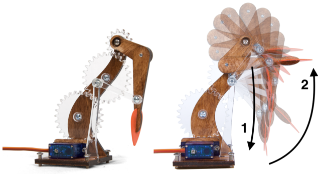
Figure 2: Left – One of the kinetic plucking mechanisms. Right – A composite image showing how the mechanism moves. The guitar pick (1) slowly plunges down next to the string, and then (2) rapidly plucks it with an upward flicking motion. The crank moves clockwise.
